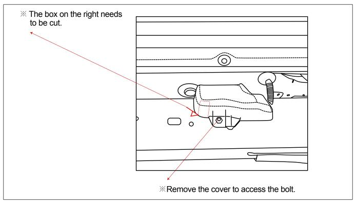
XThe inside of the driver's side. X Move the brake lines in order for the cover to come out. X Remove the cover to slip in the large nut plate.
